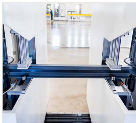
THE FOUR MITRE SAW MAKE END MILLING SYNCHRONOUSLY
